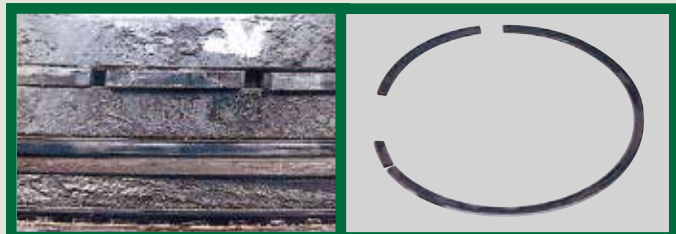
Piston Ring Breakage Caused by Excessive Piston Groove Wear
