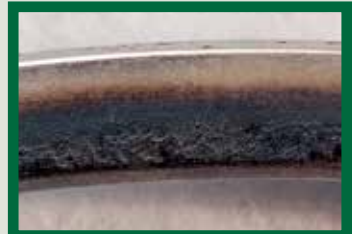
Accumulated Carbon Deposit on Piston Ring Side face
