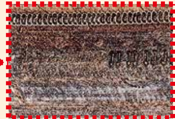
Chain Marks Due to Foreign Particles on Piston Ring Side Face
