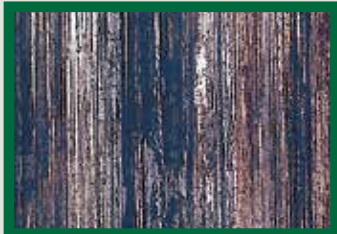
Scuffed Running Face of Piston Ring
