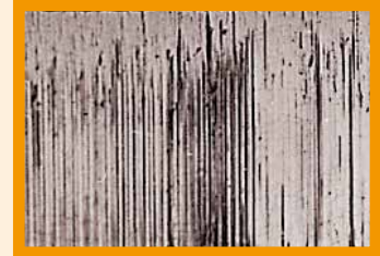
Scratch Marks on Piston Ring Running Face Caused By Foreign Particles
