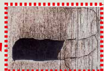
Piston Ring Breakage Caused by Excessive Piston Groove Wear
